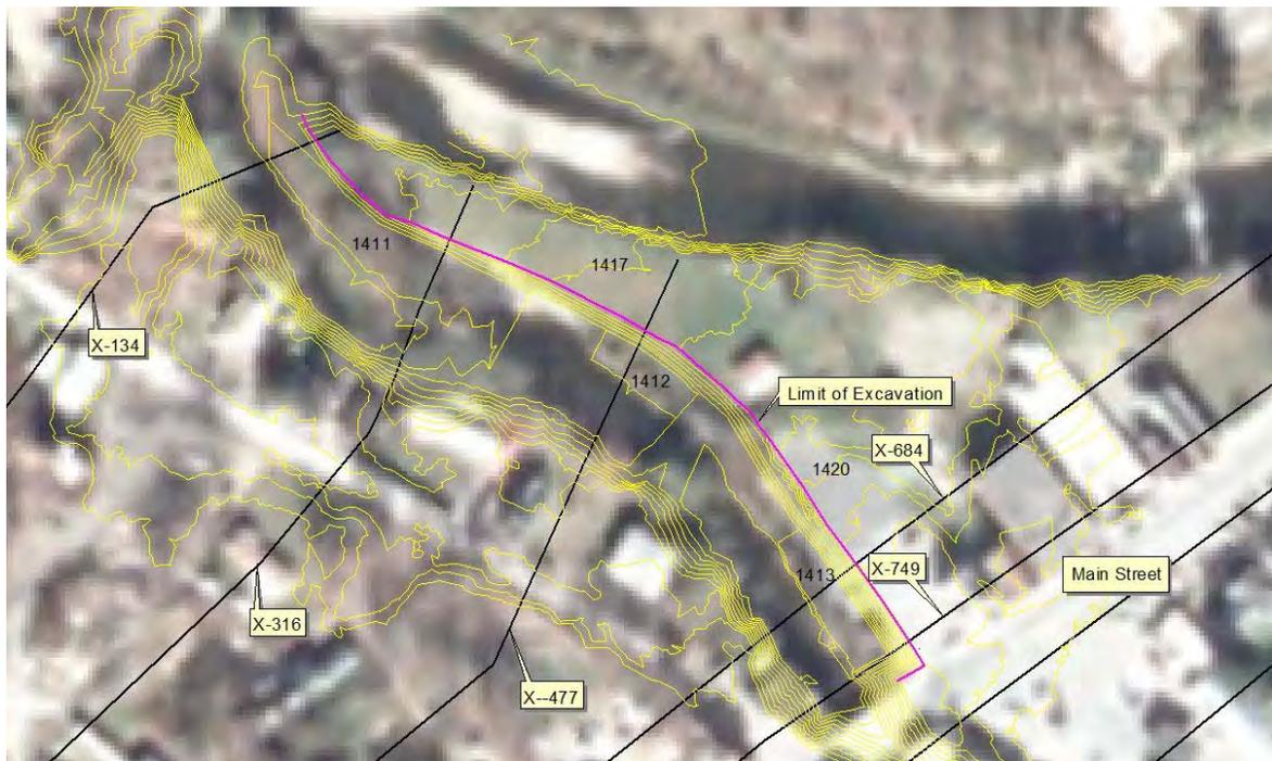
**Figure 4.3: Plan view of streambank bench along Little Beaver Kill downstream of Main St. Bridge.**
